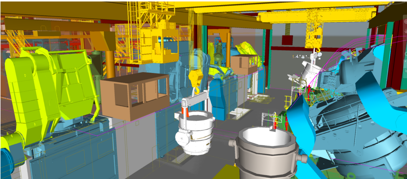
AMERICAN Cast Iron Pipe Company's Next Generation Melt Project will replace its current single cupola furnace with four coreless induction furnaces, as shown in this rendering
