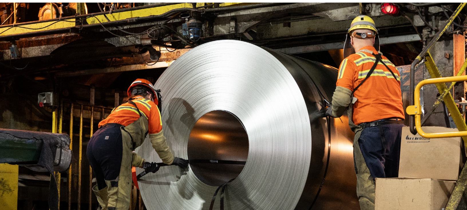
Middletown Works employees band finished steel coils
