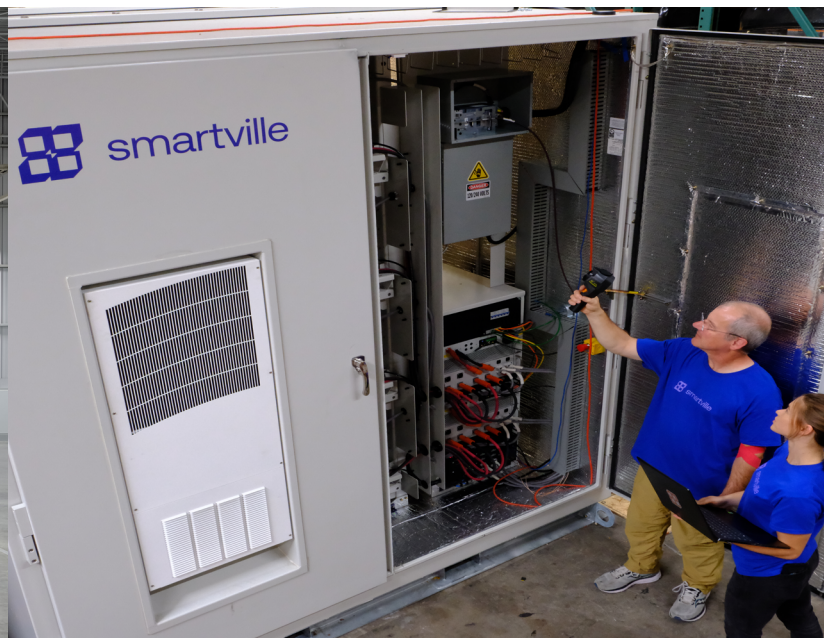
Smartville engineers conduct a quality control check on a Smartville 360 energy storage system. The energy storage system features second-life electric vehicle battery packs integrated with proprietary power electronics and controls, enhancing system reliability and extending its useful life.
